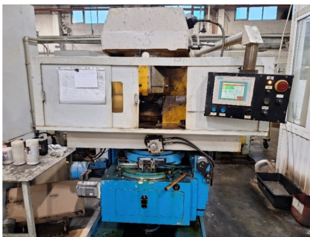
Figure 2 – Gear cutting machine. Model BCH-732NC22-7745
