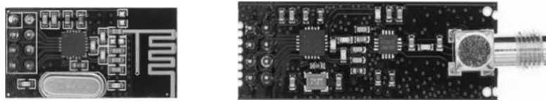
Figure 1 - NRF24L01+ and NRF24L01+PA+LNA transceivers
