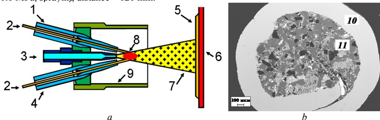
1 – cathode; 2 – PW; 3 – compressed air; 4 – anode; 5 – coating; 6 – substrate; 7 – molten metal;
