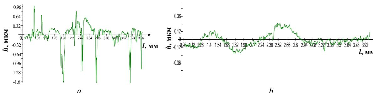
Figure 3 – Surface profiles of EACs made of Cr6B3Al6 CW with a roughness of  $Ra$  1.88 (*a*) and steel 100Cr1,5 with a roughness of  $Ra$  0.88 (*b*) after grinding and polishing. The ordinate axis shows the difference in relief heights on the surfaces,  $\mu\text{m}$ , and the abscissa axis shows the length of the path along which the measurements were made,  $\mu\text{m}$ .
