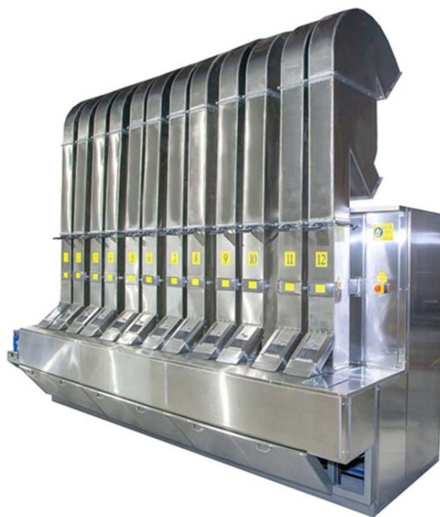
Figure 4 – General view of the experimental research prototype of the column-type aerodynamic separator SS-012 (LLC «RPA Sorting Machines»).
